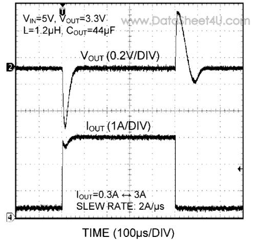
FIGURE 9. Load Step Response without  $C_{FF}$
