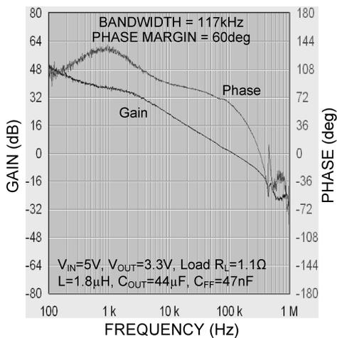
FIGURE 8. Loop Gain and Phase with  $C_{FF}$
