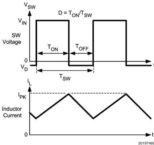
FIGURE 2. Typical Waveforms
