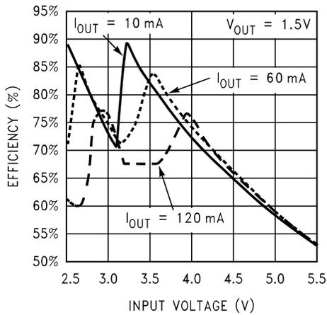
Efficiency vs. Output Current: LM2788-1.5
