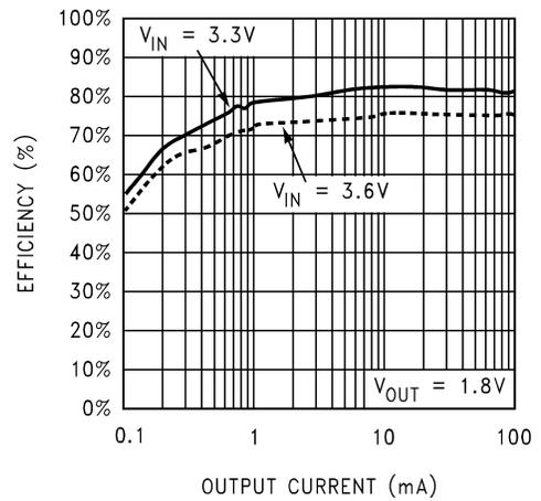
Efficiency vs. Input Voltage: LM2788-2.0
