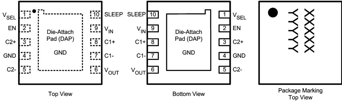
**Note:** The actual physical placement of the package marking will vary from part to part. The package marking placeholder "XXXXX" is a code for die traceability. "YYYYY" identifies the device (part number, voltage option, etc.). See the Order Information table below for device ID codes.
