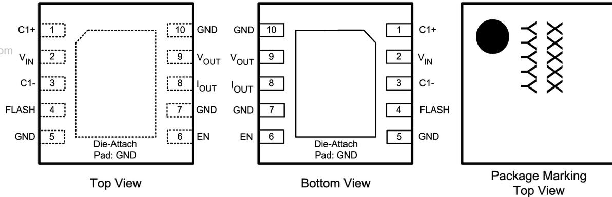
**Note:** The actual physical placement of the package marking will vary from part to part. The package marking placeholder "XXXXX" is a code for die traceability. "YYYYY" identifies the device (part number, voltage option, etc.). See the Order Information table below for the device ID codes.
