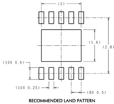
DIMENSIONS ARE IN MILLIMETERS
