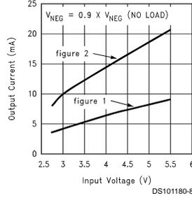
**No Load Supply Current vs. Input Voltage**
