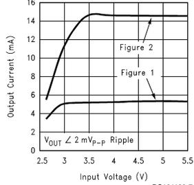
**Maximum  $V_{NEG}$  Current vs. Input Voltage**
