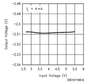
**Typical Performance Characteristics** Unless otherwise specified,  $T_A = 25^\circ\text{C}$ ,  $V_{OUT} = -2.5\text{V}$ . (Continued)
