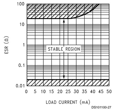
**FIGURE 6. ESR Curve for  $C_{OUT} = 10\mu F$**
