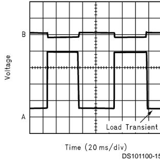
A: LOAD CURRENT:  $I_{LOAD} = 5\text{mA to } 39.6\text{mA}$ , 10mA/div
