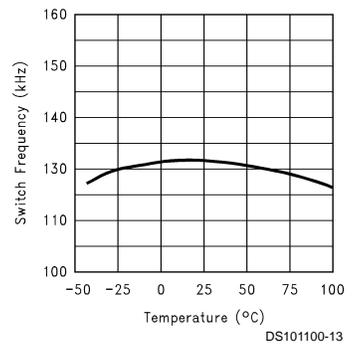
**Typical Performance Characteristics** Unless otherwise specified,  $T_A = 25^\circ\text{C}$ ,  $V_{IN} = 3.6\text{V}$ . (Continued)
