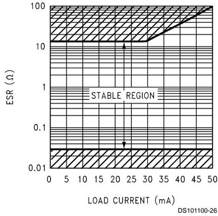
**FIGURE 5. ESR Curve for  $C_{OUT} = 4.7\mu F$**
