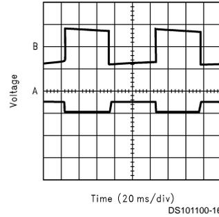
A: LOAD CURRENT:  $I_{LOAD} = 4.4\text{mA to } -9.4\text{mA}$ , 10mA/div
