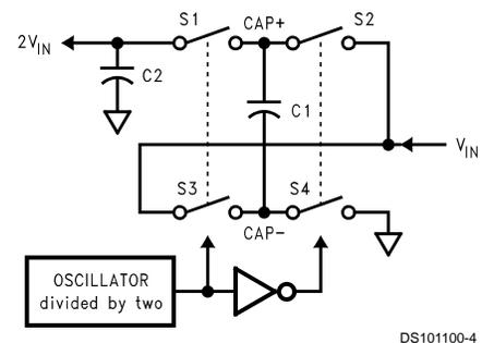
FIGURE 2. Voltage Doubler Principle
