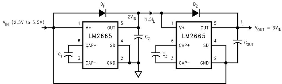
FIGURE 4. Increasing Output Voltage by Cascading Devices
