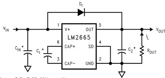
\*  $C_{IN}$ ,  $C_1$ , and  $C_2$  are  $3.3 \mu\text{F}$  OS-CON capacitors.
