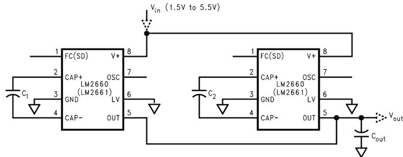
FIGURE 4. Lowering Output Resistance by Paralleling Devices
