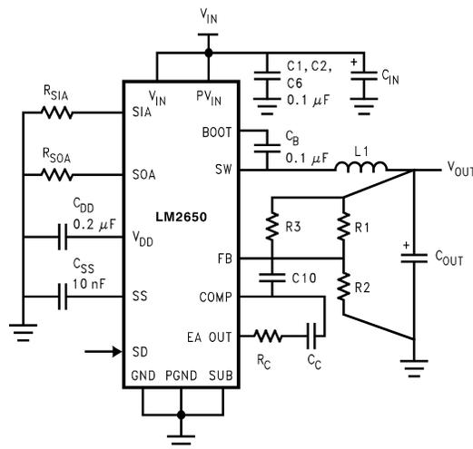
FIGURE 4. The Typical 90 kHz Application Circuit
