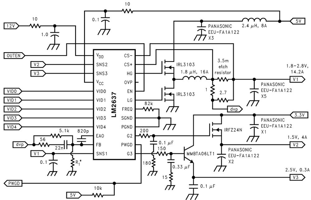
\*  $R_1$  is for raising the switcher output voltage slightly. Its value depends on the output voltage.
