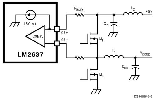
FIGURE 4. Current Limit via High-Side FET  $V_{DS}$  Sensing
