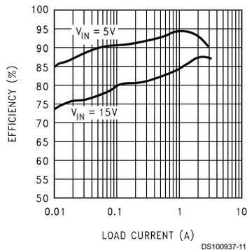
**Efficiency (FPWM = High, Input Voltage = 16V**
