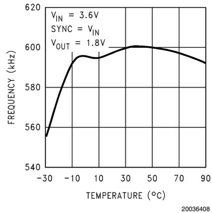
**Typical Operating Characteristics** LM2618ATL, Circuit of *Figure 1*,  $V_{IN} = 3.6V$ ,  $T_A = 25^\circ C$ ,  $L_1 = 10 \mu H$ , unless otherwise noted. (Continued)
