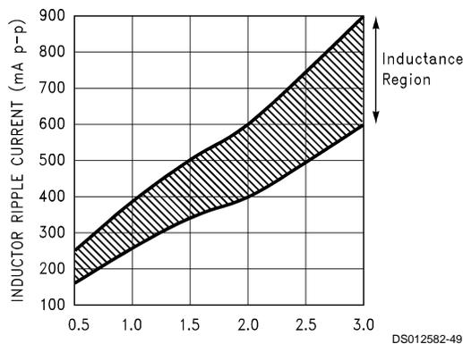
**FIGURE 20. Peak-to-Peak Inductor Ripple Current vs Load Current**
