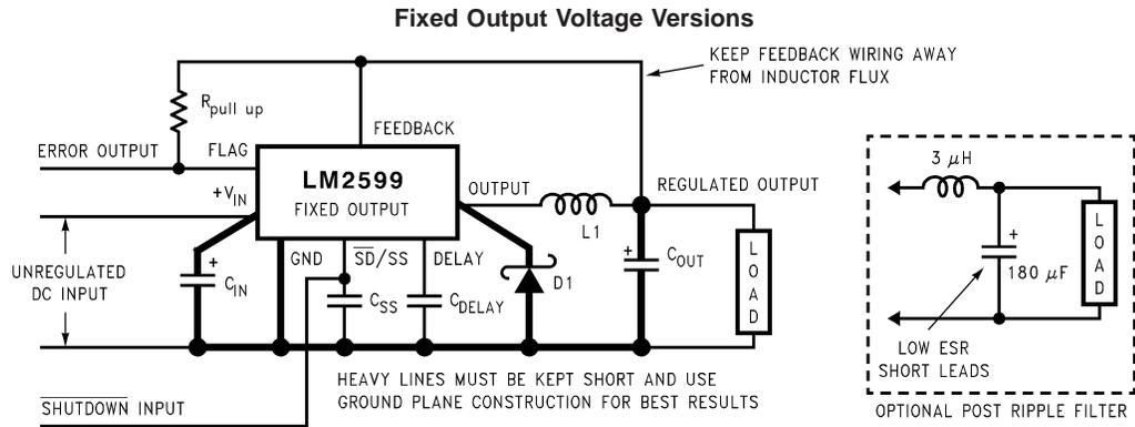
Component Values shown are for  $V_{IN} = 15V$ ,
