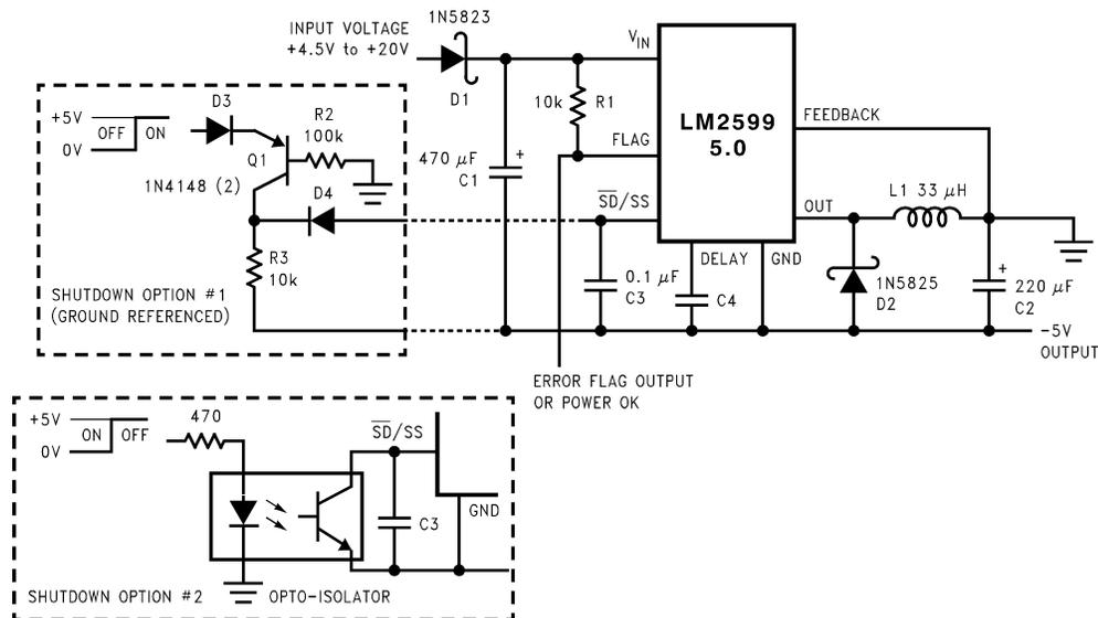
FIGURE 26. Inverting -5V Regulator With Shutdown and Soft-start
