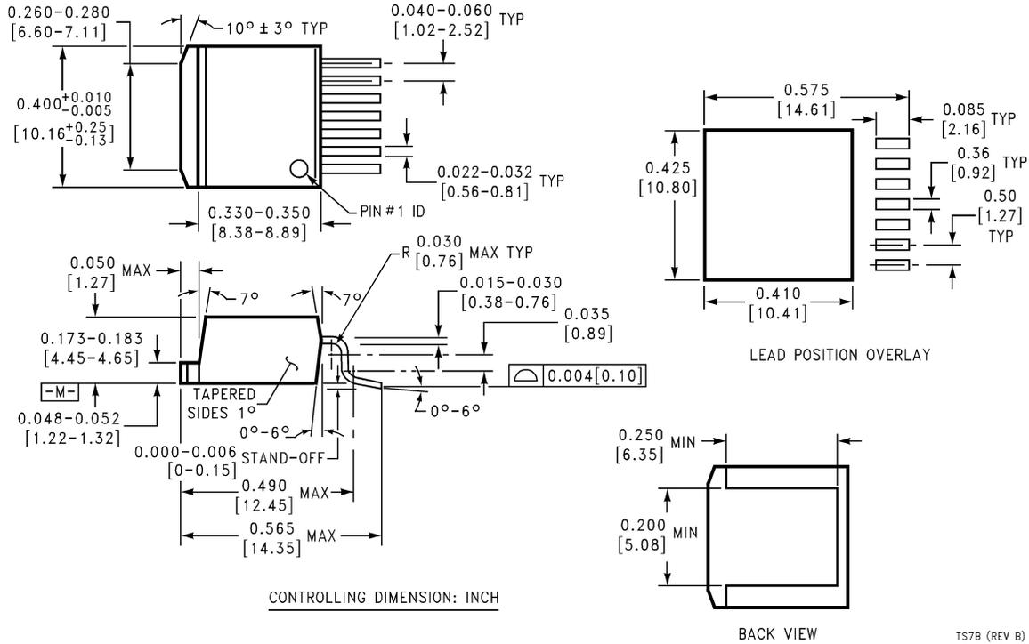
**7-Lead TO-263 Bent and Formed Package**
