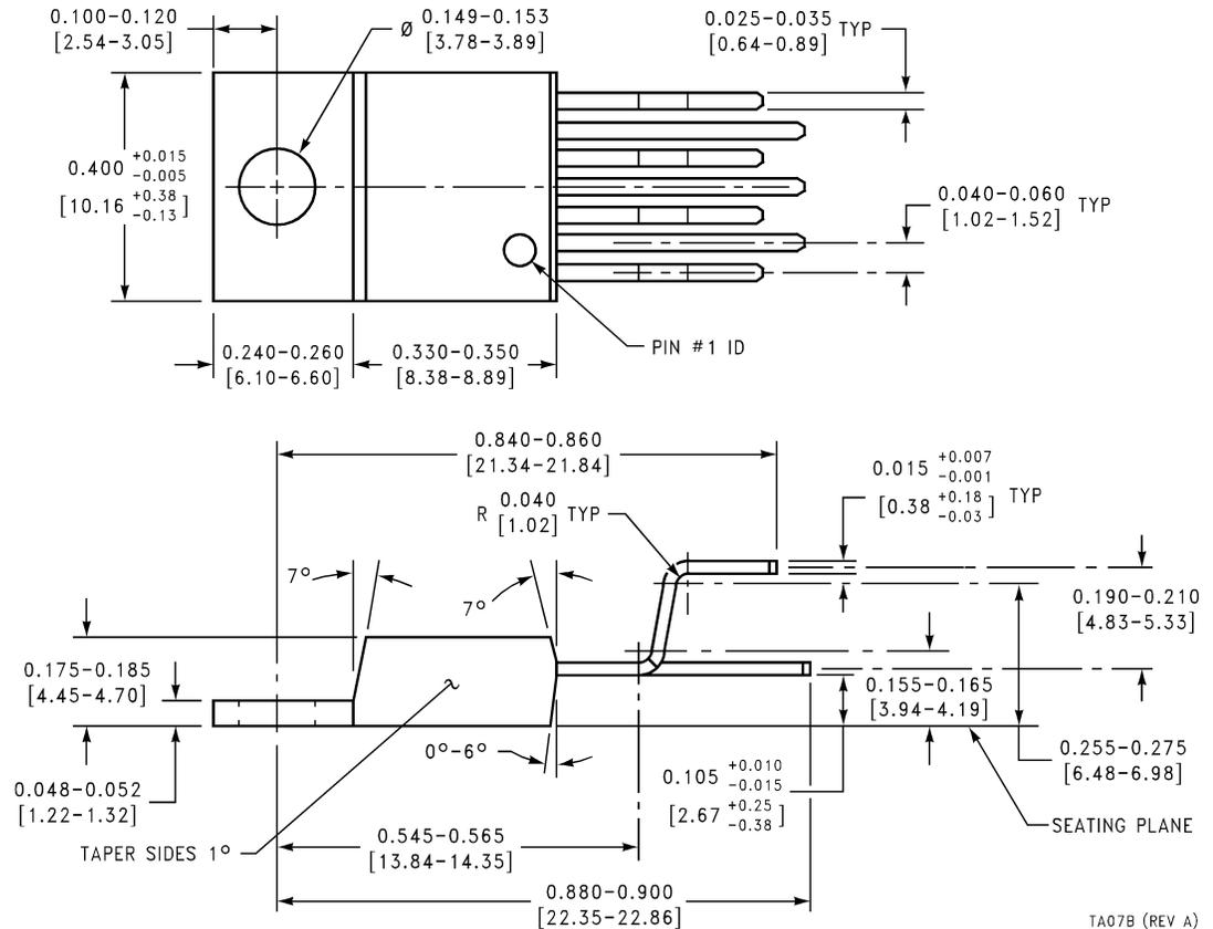
**7-Lead TO-220 Bent and Staggered Package**
