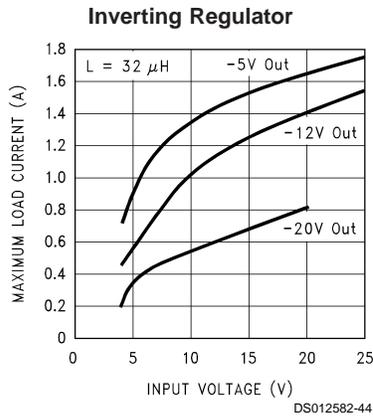
**FIGURE 27. Maximum Load Current for Inverting Regulator Circuit**
