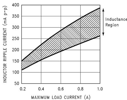
**FIGURE 20. Peak-to-Peak Inductor Ripple Current vs Load Current**
