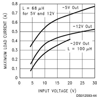
**FIGURE 27. Maximum Load Current for Inverting Regulator Circuit**
