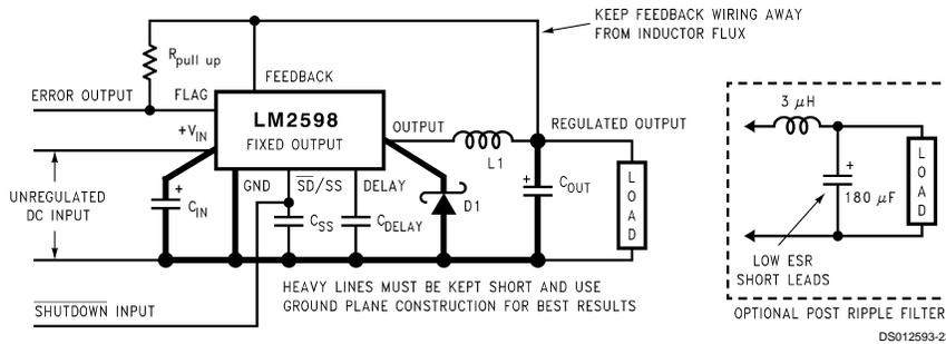
Component Values shown are for  $V_{IN} = 15V$ ,  $V_{OUT} = 5V$ ,  $I_{LOAD} = 1A$ .
