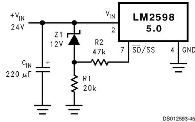
**FIGURE 28. Undervoltage Lockout for a Buck Regulator**
