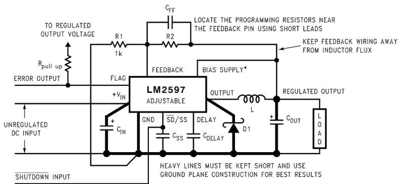
$$V_{OUT} = V_{REF} \left( 1 + \frac{R_2}{R_1} \right) \quad \text{where } V_{REF} = 1.23V$$
