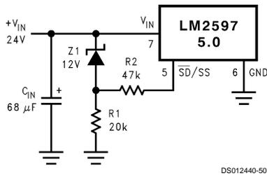
**FIGURE 30. Undervoltage Lockout for a Buck Regulator**
