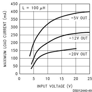
FIGURE 29. Maximum Load Current for Inverting Regulator Circuit
