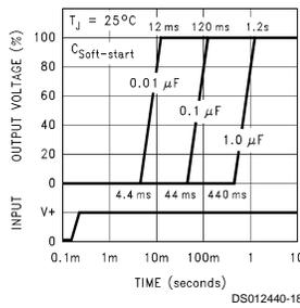
**Shutdown /Soft-start Threshold Voltage**
