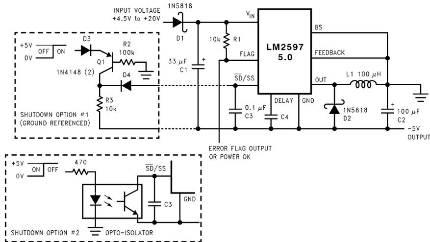
FIGURE 28. Inverting -5V Regulator With Shutdown and Soft-start
