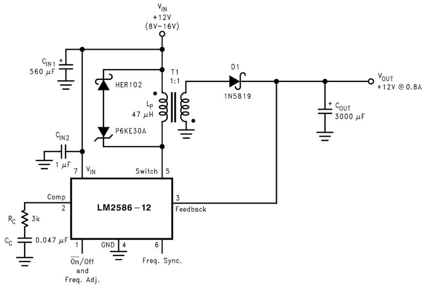
As shown in Figure 4, the LM2586 can be used as a flyback regulator by using a minimum number of external components. The switching waveforms of this regulator are shown in Figure 5. Typical Performance Characteristics observed during the operation of this circuit are shown in Figure 6.
