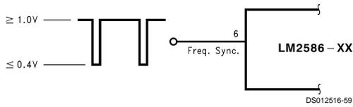
FIGURE 40. Frequency Synchronization
