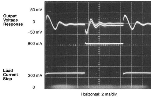
FIGURE 6.  $V_{OUT}$  Response to Load Current Step
