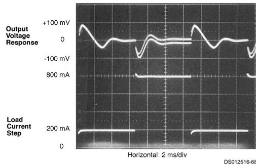
FIGURE 32.  $V_{OUT}$  Response to Load Current Step
