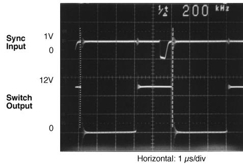
FIGURE 41. Waveforms of a Synchronized 12V Boost Regulator
