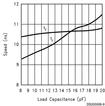
Figure 14: Speed vs Load Capacitance
