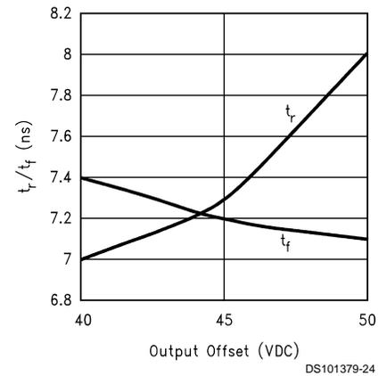
FIGURE 9. CRT Driver Speed vs. Offset
