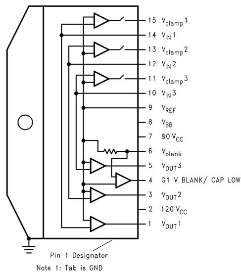
FIGURE 2. LM2457 Package Pinout
