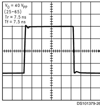
FIGURE 7. CRT Driver Transient Response
