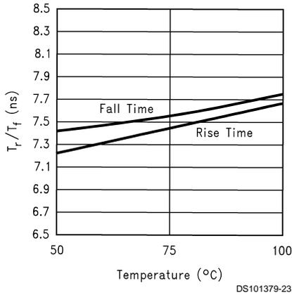
FIGURE 6. CRT Driver Speed vs. Temperature
