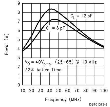
FIGURE 8. CRT Driver Power Dissipation vs. Frequency
