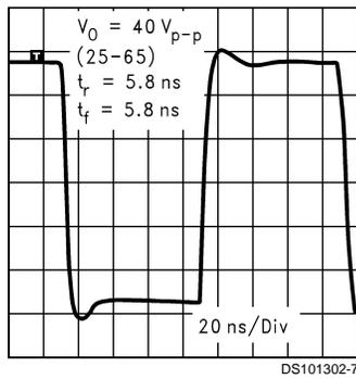
**FIGURE 7. CRT Driver Transient Response**
