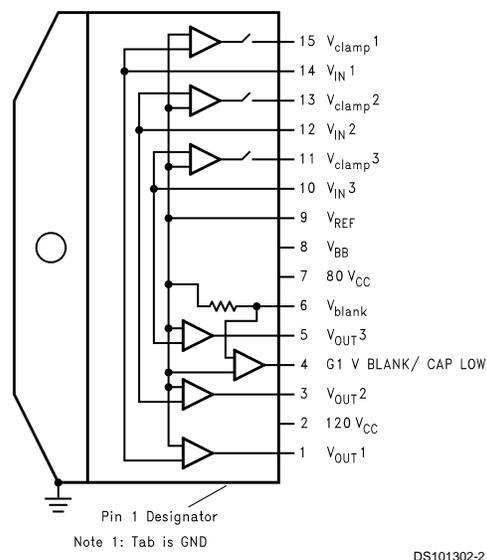
FIGURE 2. LM2453 Package Pinout
