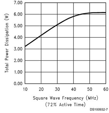
FIGURE 6. Power Dissipation vs Frequency (72% Active Time)
