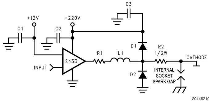
FIGURE 12. Recommended Application Circuit
