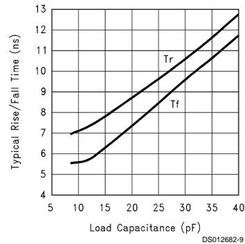
FIGURE 8. Effect of Load Capacitance on Rise/Fall Time
