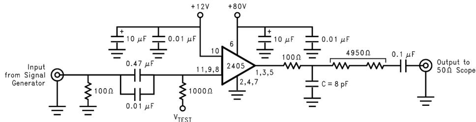
**Note:** 8 pF is total load plus parasitic capacitance.
