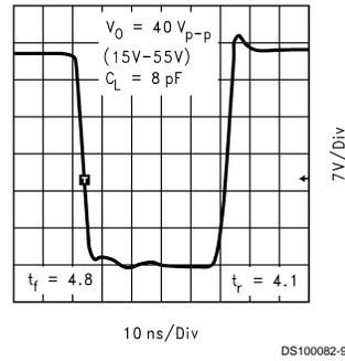
FIGURE 8. Pulse Response with  $V_{CC} = 70$  V<sub>DC</sub>
