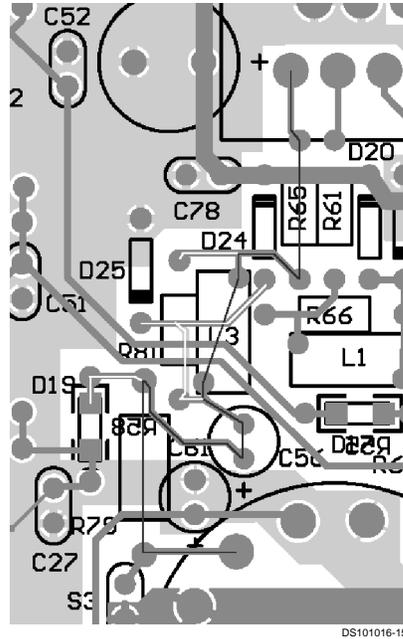
FIGURE 13. PCB CRT Driver, Blue Channel Output
