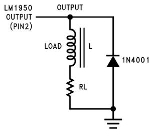
FIGURE 2. Diode Clamp
