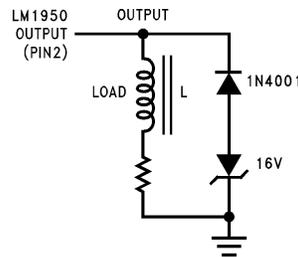
FIGURE 3. Zener Clamp for Rapid Controlled Current Decay
