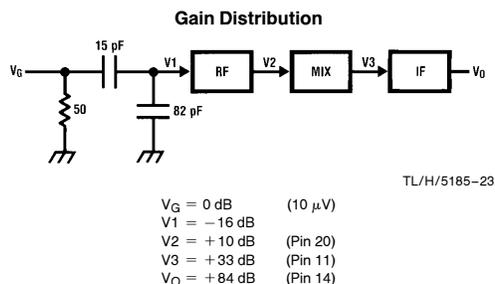
The IF gain could also be varied by changing the value of R6 across the IF output coil. However, it is a good idea to maintain a high Q IF tank in order to achieve good adjacent channel rejection. In order to prevent distortion due to overloading the IF amplifier, it is important that the impedance Pin 14 sees looking into the IF output tank, T5, does not go below 3K ohms.
