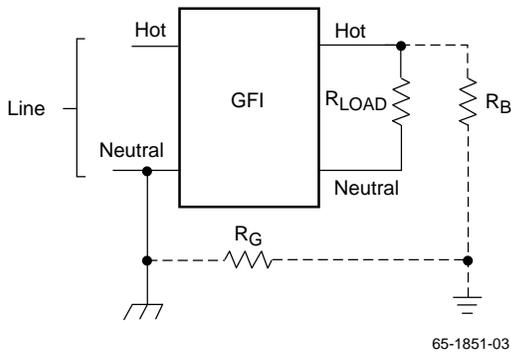
Figure 1. Normal Fault
