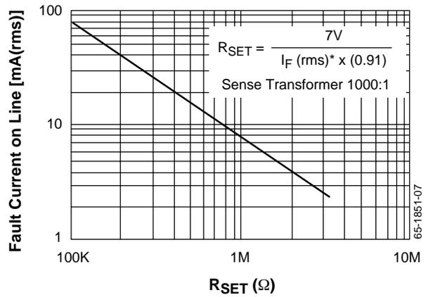
Figure 5. Normal Fault Current Threshold vs. RSET
