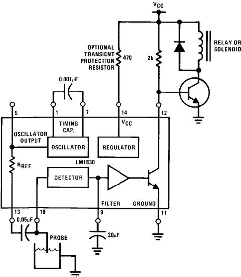
The Output is suitable for driving a sump pump or opening a drain valve, etc.
