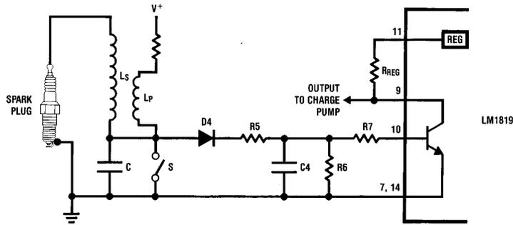
FIGURE 5. Typical Pulse-Squaring Circuit for Automotive Tachometers.
