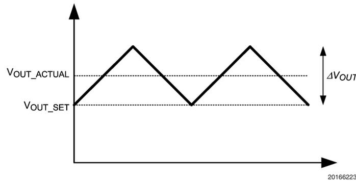
It can be seen that the average output voltage ( $V_{OUT\_ACTUAL}$ ) is higher than the output voltage ( $V_{OUT\_SET}$ ) that was calculated by the earlier equation by exactly half the output voltage ripple. The output voltage that is targeted for regulation may then be appended according to the voltage ripple. This can be seen below:
