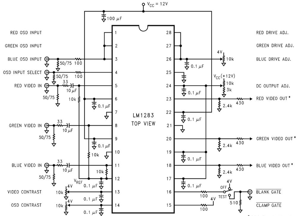
\* 50 $\Omega$  Termination to be Used at Outputs
