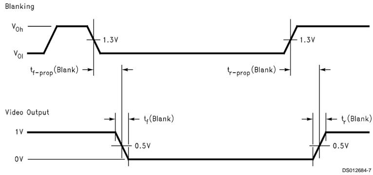
FIGURE 2. Blanking Propagation Delay and Rise/Fall Time
