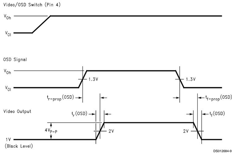
FIGURE 4. OSD Propagation Delay and Rise/Fall Times
