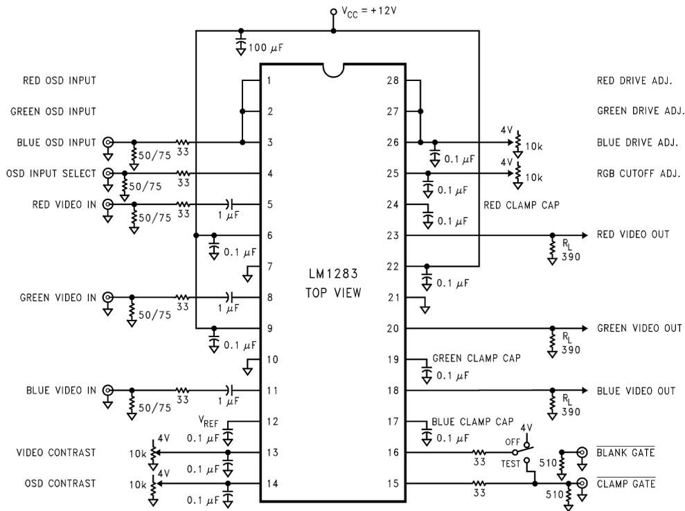
FIGURE 5. LM1283 OSD Video Preamp DC Test Circuit
