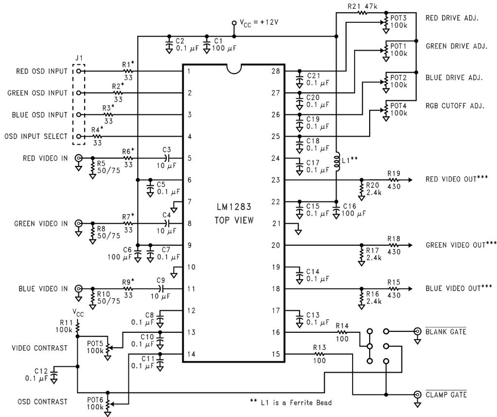
\*Note: All video inputs must have a series 33Ω resistor for protection against EOS (Electrical Over Stress). If the OSD input signals are external to the monitor, or these signals are present any time when +12V is not fully powered up, then the OSD inputs also require a series 33Ω resistor.
