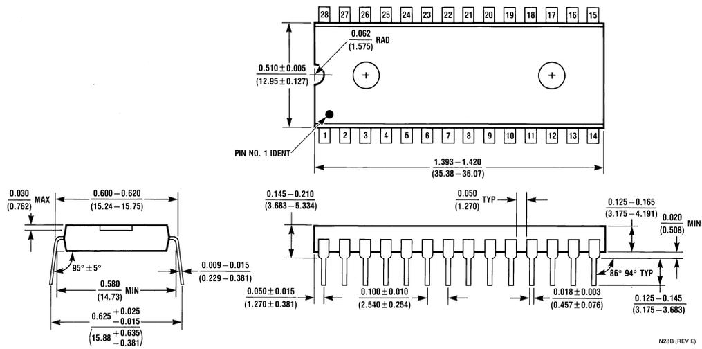
**28-Lead (0.600" Wide) Molded Dual-In-Line Package
