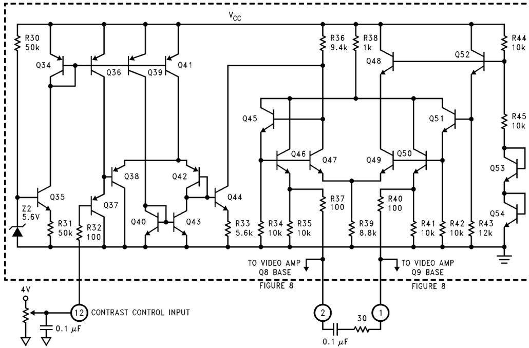
FIGURE 9. Simplified Schematic of LM1208/LM1209 Contrast Control
