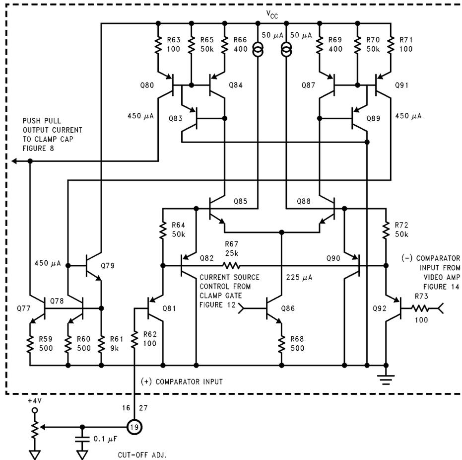
FIGURE 11. Simplified Schematic of LM1208/LM1209 Clamp Comparator Circuit
