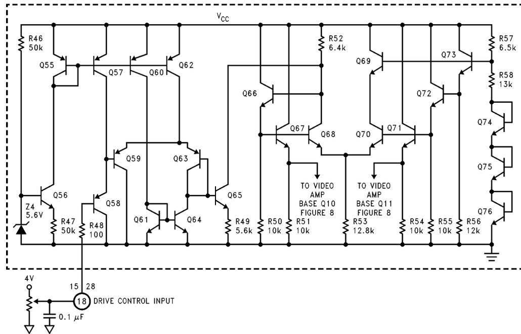
FIGURE 10. Simplified Schematic of LM1208/LM1209 Drive Control
