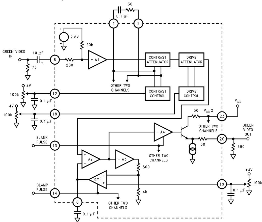
FIGURE 6. Block Diagram of LM1208/LM1209 Video Amplifier
