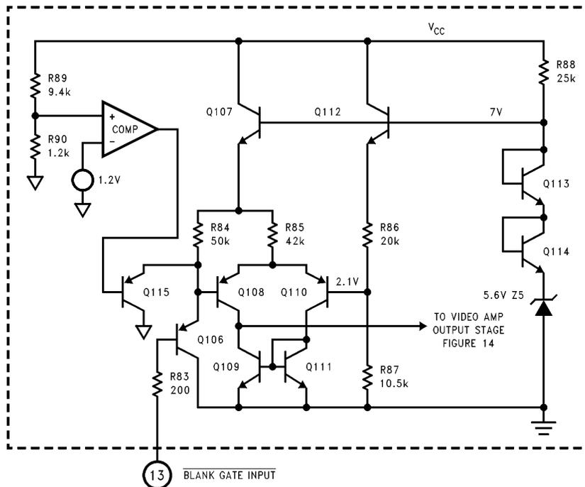
FIGURE 13. Simplified Schematic of LM1208/LM1209 Blank Gate Circuit
