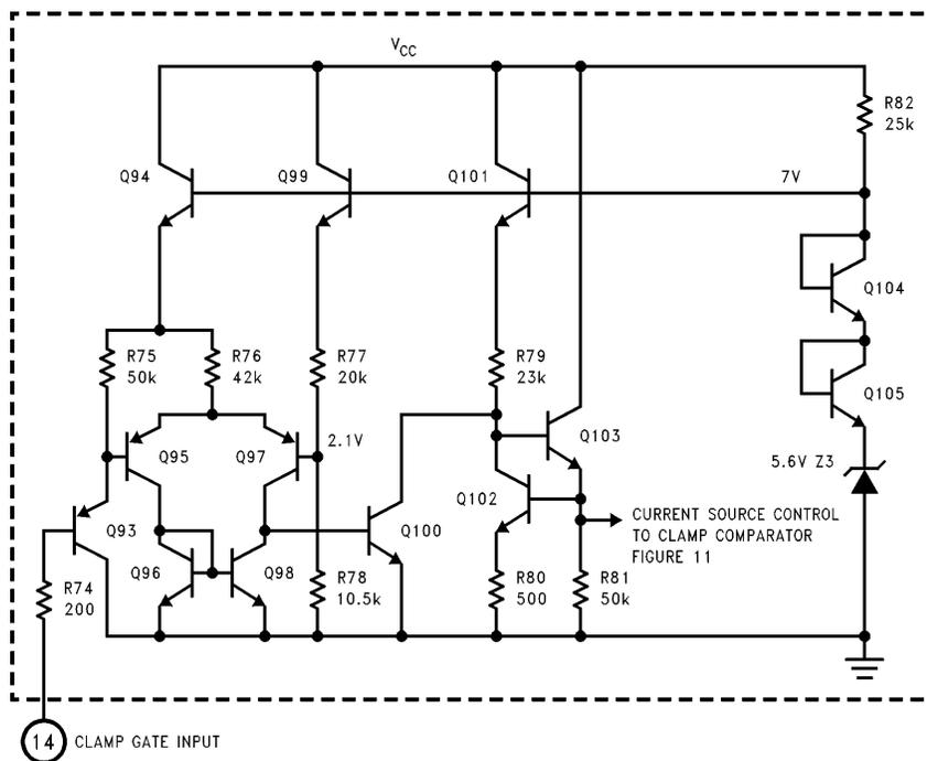
FIGURE 12. Simplified Schematic of LM1208/LM1209 Clamp Gate Circuit
