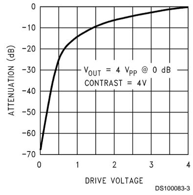
**Typical Performance Characteristics**  $V_{CC} = 12V$ ,  $T_A = 25^\circ C$  unless otherwise specified (Continued)
