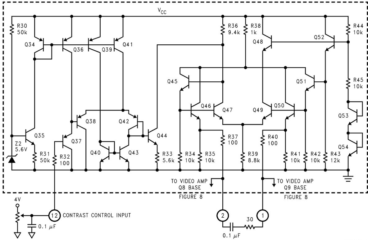
FIGURE 9. Simplified Schematic of LM1208 Contrast Control
