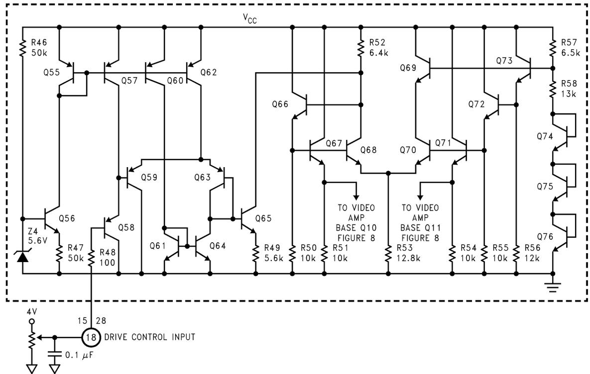
FIGURE 10. Simplified Schematic of LM1208 Drive Control
