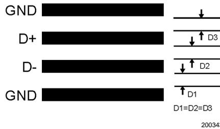
**FIGURE 6. Recommended Diode Trace Layout**
