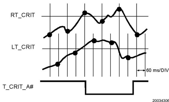
FIGURE 3.  $\overline{T\_CRIT\_A}$  Temperature Response Diagram
