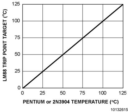
**FIGURE 3. Pentium or 3904 Temperature vs LM88 Temperature Set-point**
