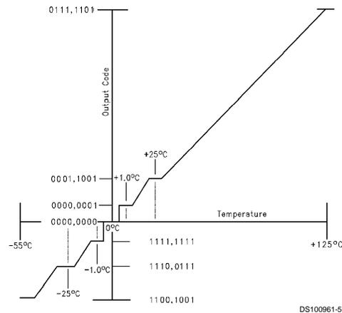
FIGURE 2. Temperature-to-Digital Transfer Function (Non-linear scale for clarity)
