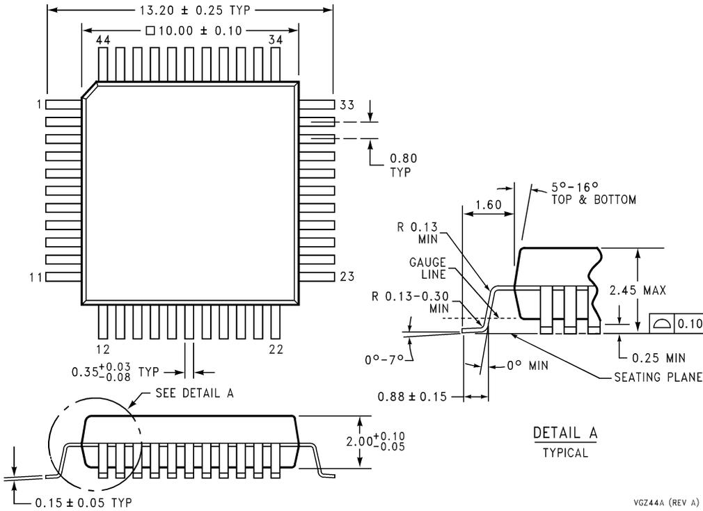
**44-Lead (10 mm x 10 mm) Molded Plastic Quad Flatpak**
