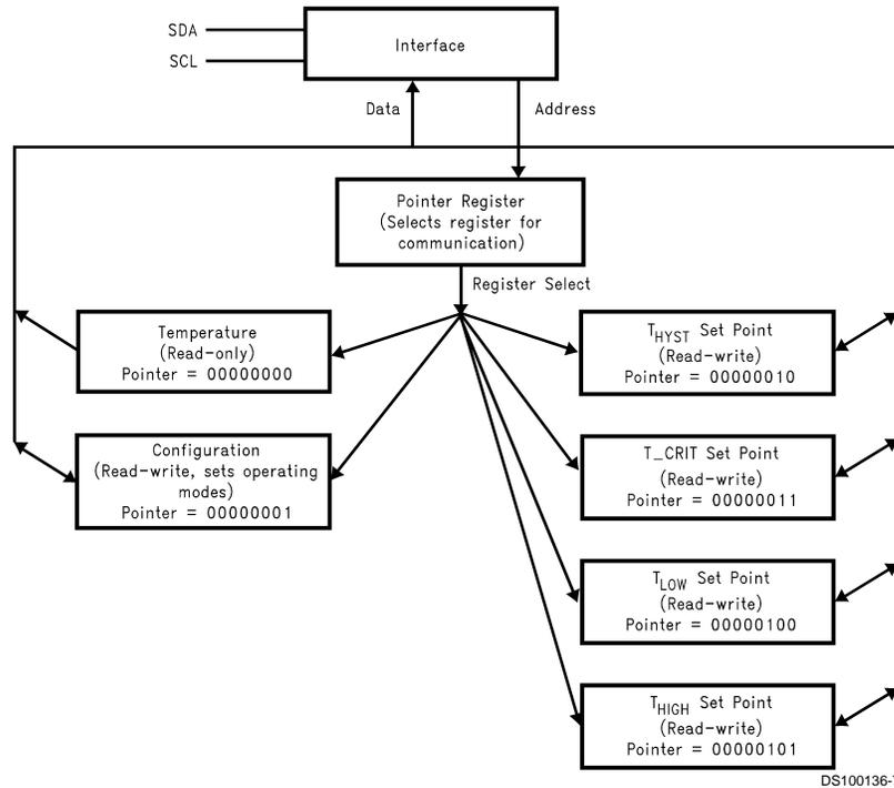
There are four data registers in the LM77, selected by the Pointer register. At power-up the Pointer is set to "00"; the location for the Temperature Register. The Pointer register latches the last location it was set to. In Interrupt Mode, a read from the LM77 resets the INT output. Placing the device in Shutdown mode resets the INT and T\_CRIT\_A outputs. All registers are read and write, except the Temperature register which is read only.
