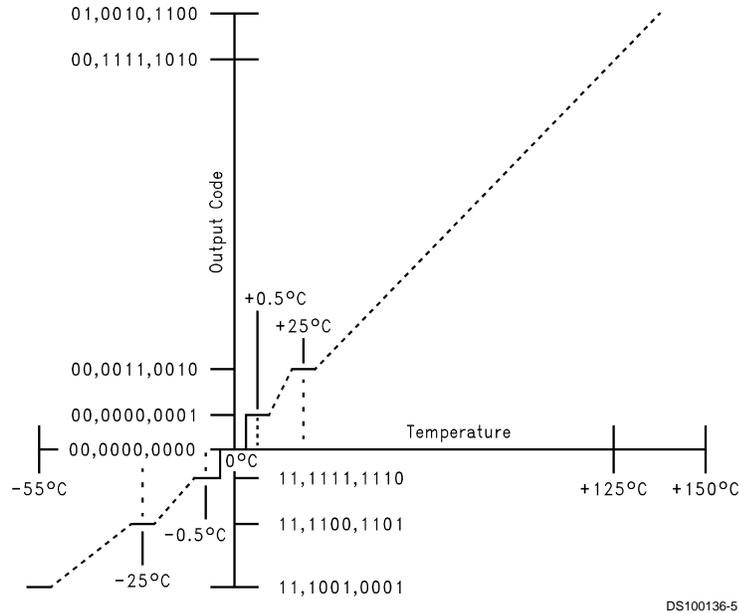
FIGURE 2. Temperature-to-Digital Transfer Function (Non-linear scale for clarity)
