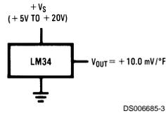
**FIGURE 1. Basic Fahrenheit Temperature Sensor (+5° to +300°F)**
