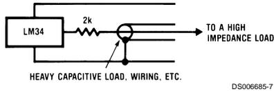
FIGURE 3. LM34 with Decoupling from Capacitive Load
