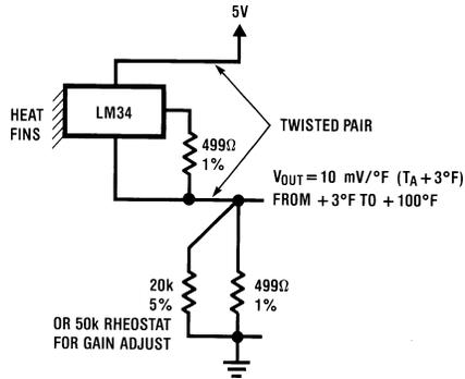
$V_{OUT} = 10\text{mV}/^{\circ}\text{F} (T_A + 3^{\circ}\text{F})$
