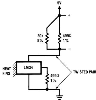
$V_{OUT} = 10\text{mV}/^{\circ}\text{F} (T_A + 3^{\circ}\text{F})$
