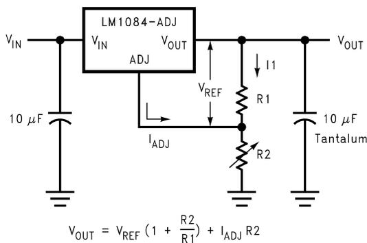
$$V_{OUT} = V_{REF} \left( 1 + \frac{R_2}{R_1} \right) + I_{ADJ} R_2$$
